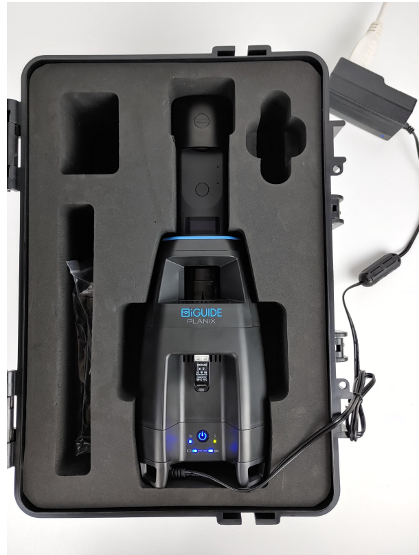
Figure 5 - Charging, PLANIX turned on
